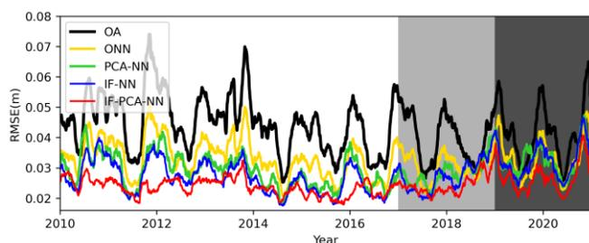
Fig. 6. The time series of the spatial average over region A of the RMSEs of SSH among the three experiments (unit: m; OA method, black line; ONN method, yellow line; PCA-NN method, green line; IF-NN method, blue line; IF-PCA-NN, red line). Lightly shaded is the period over which the validation set is formed, and the period with dark shading is for test set.
