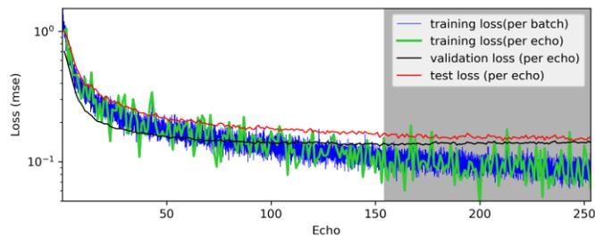
Fig. 5. The evolution of the loss functions for the first PC with different sets. The blue line indicates the training set (per batch), while the green, red, and black lines are for the training, validation, and testing sets, respectively (per echo).
